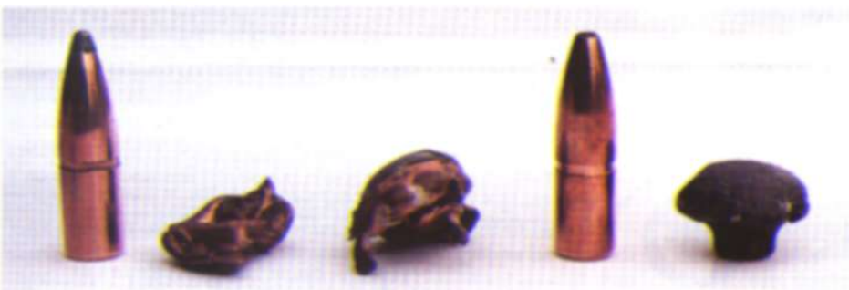
Recovered bullets – left to right: 220gr Hornady new as comparison; recovered from zebra; recovered from wetpack. 220gr Swift (new) and from wetpack.
