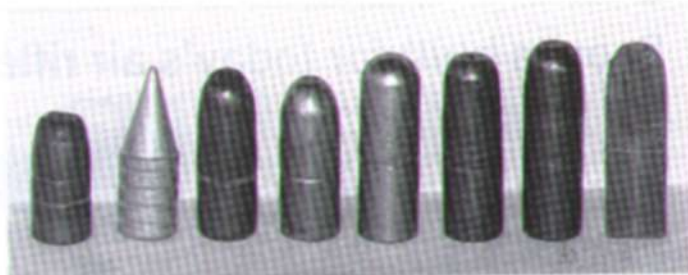
Above: Bullets used in the tests (from left) 400gr Speer Flat Nose; 300gr Impala; 500gr Hornady SP; 500gr Claw SP; 475gr PMP Monolithic; 500gr Rhino Solid Shank; 550gr Rhino SS; same bullet sectioned. Left: (L-r) .416 Rigby; .458 Winchester Magnum; .460 Weatherby Short; .458 Lott; .450 Ackley; .450 Rigby Rimless Magnum; .460 Weatherby.
