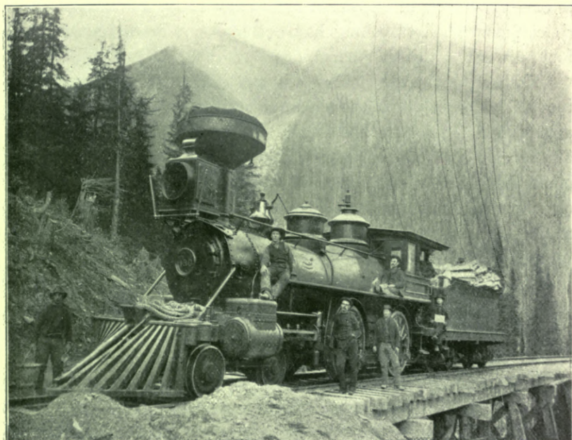
A "MOGUL" LOCOMOTIVE, USED BY THE C. P. RAILWAY TO CROSS THE SELKIRK MOUNTAINS, KOOTENAY, B.C.
