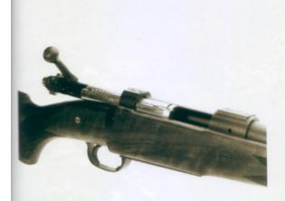
Mauser and Winchester systems do. It is a better system from this point of view. The ejector pin is sturdy and, since ejection is manual and at the rear of the bolt stroke, the Express offers the advantages of the Mauser system without the shortcomings of the modified modern Mauser designs. Its cartridges will stay in line until ejected and short stroking and double feeding is inhibited. As reliable a system as any with gas flow advantages.
