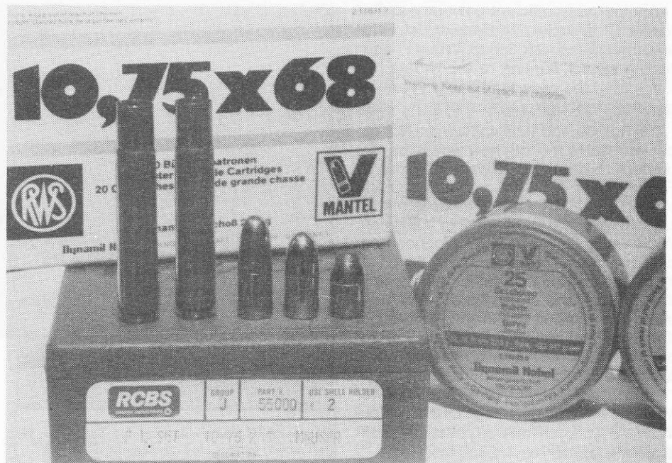
RCBS Group J dies were used to re-load the 10.75 x 68. Their high polish made life easy for the operator.
