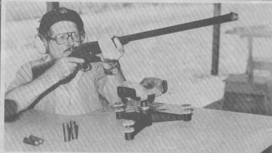
The 12-bore "Jungle Gun" was a proprietary patent of Army & Navy Co-operative Stores, manufactured by Webley & Scott. From a bench the recoil is considerable from the 800-gr. Paradox load of 5 drams of Fg. The rifling only twists 2 1/2 inches from the muzzle to increase stability.
