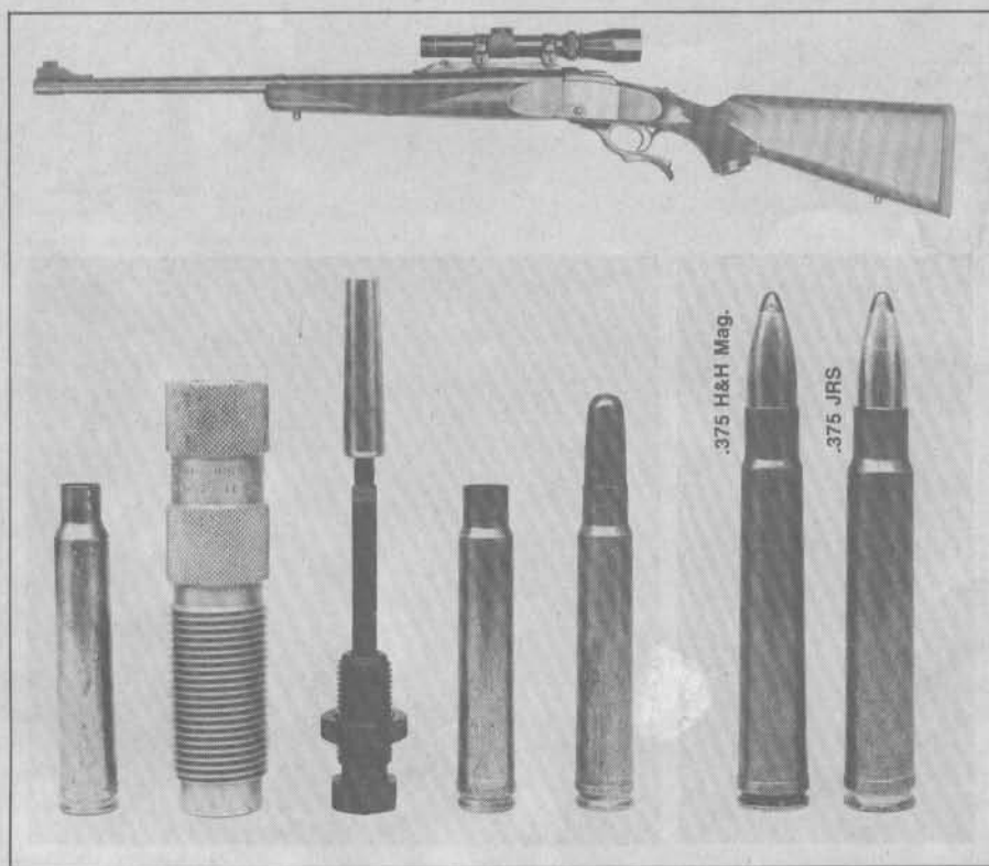
G&A Eastern Field Editor Jon R. Sundra devised his own .375 JRS wildcat based on the 8 mm Remington Magnum case necked up to .375 for use in his rechambered Ruger No. 1 (top). Cases can be formed by necking up 8 mm Rem. Mag. brass with a long tapered expander (above left) or by fire-forming .375 H&H Mag. factory rounds. The .375 JRS (left) is very similar to several other "improved" .375 Magnums.
