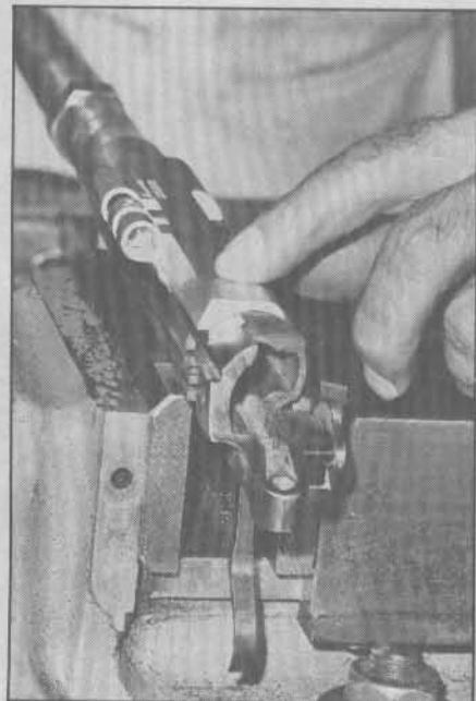
For scope mounting on the author's experimental .475 LTD rifle built on an Enfield action, a Pachmayr Lo-Swing mount was milled to fit the receiver.
