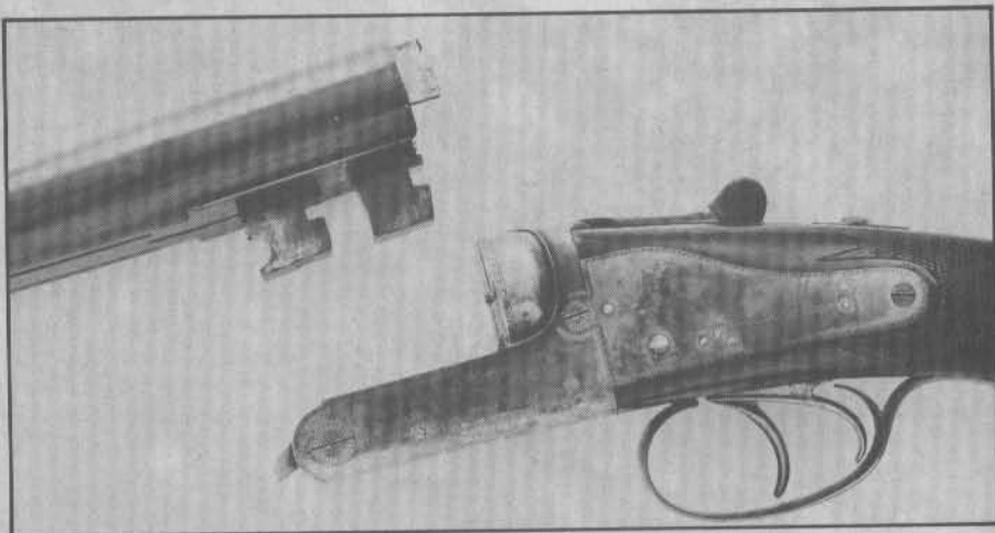
On smokeless powder doubles like this Holland & Holland Number 2 Grade, the barrel lugs are made from integral forgings with the barrels and brazed together. They contain the slots for the sliding underbolts and the hook for the hinge pin.
