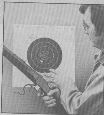
The Browning Single Shot, made in Japan, was closely patterned after the old Winchester High Wall design. This fine rifle has recently been discontinued.
