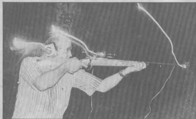
John Wootters taped flashlight bulbs to eyeglass frames and the muzzle and scope of his wildcat .416 Taylor to illustrate the effects of magnum recoil. The recoil of his 400-grain load at about 2,400 fps in this rifle amounts to about 44 foot-pounds. Here Wootters has fired and returned to position after recoil drove him through its arc.
