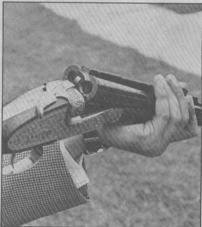
A best-grade double rifle like this Holland & Holland "Royal" Grade represents the apogee of the gunmaker's art, with its carefully regulated barrels, ultra-precise fitting of the lockwork and other contact surfaces and its exquisite engraving.
