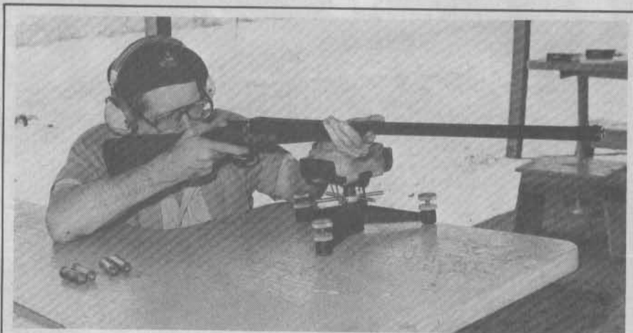
A typical working 8-bore is this J.B. Rodda back action hammer double rifle. This specimen features the underlever screw grip system and sports 22-inch .875 barrels. Built circa 1885, this 17 pound workhorse chambers brass cases.
