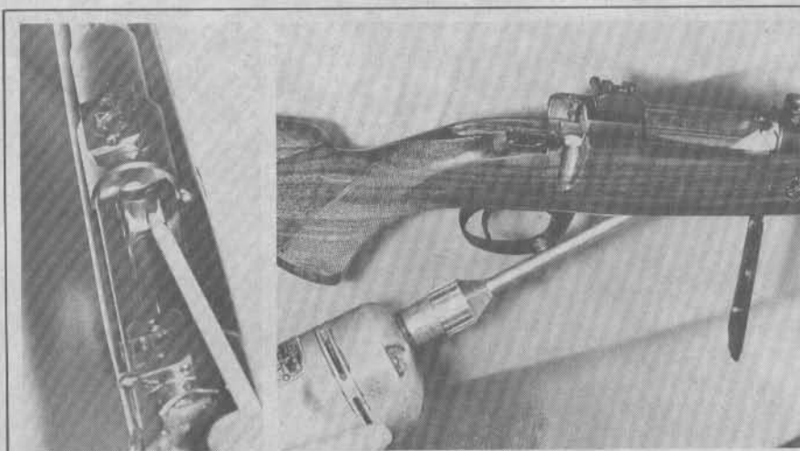
Whether your big bore is factory or custom, your life may depend on its smooth, reliable functioning! Even the best rifles may require a little polishing on the feed ramp for added smoothness. This Browning was rebarreled from .264 to .458, requiring ramp modification, left, and polishing with an emery cloth.
