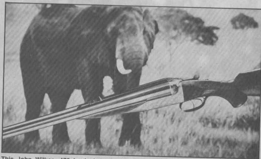
This John Wilkes .470 boxlock is the last rifle that was made for the great ivory hunter and gun authority John "Pondoro" Taylor. Although lacking some of the advantages of the sidelock, boxlocks like this were sturdy and gave excellent service.
