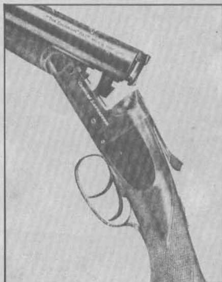
Charles Lancaster's "Colindian" double rifle was a take-off of the "Paradox"-type big bore with the unique muzzle-tip twist—but would also fire shot loads.
