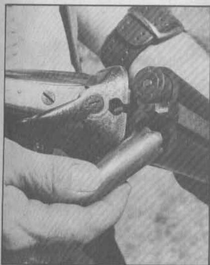
This "Jungle Gun" has a unique "doll's head" third fastener extending from the rib. The author loads an 800-gr. conical bullet housed in a 12 ga. brass case.
