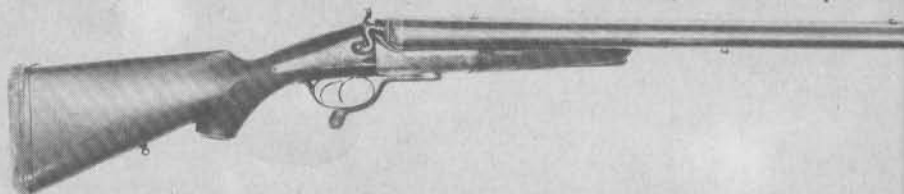
A typical working 8-bore is this J.B. Rodda back action hammer double rifle. This specimen features the underlever screw grip system and sports 22-inch .875 barrels. Built circa 1885, this 17 pound workhorse chambers brass cases.
