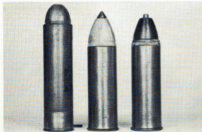
All are 8-bore: (l.) a pinfire, 3½" brass-and-paper case by Eley for a French rifle; (r.) two 2-9/16" Utendoerfer (Nuremberg) rifle cartridges loaded with a steel-pointed, explosive, lead bullet and the solid-iron, lead-belted bullet.
