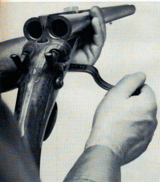
To swing the 10½-lb. barrels of the Osborne 8-bore requires practice and strength. The side-lever operates double under-bolts. Note doll's-head extension and reinforcing tang over pistol grip.
