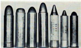
(l. to r.) 12-bore brass case with enclosed hollow-point lead bullet; 12-bore Westley Richards Explora, solid lead; 12-bore Kynoch Nitro ball; 12-bore Kynoch hollow split cap; 20-bore Pegamoid by Eley with Westley Richards brass-capped bullet; 28-bore by Eley, also with brass-capped bullet; early 24-bore rifle cartridge with paper-patched bullet.
