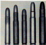
Some big-bore cartridges for which magazine rifles are chambered are (l. to r.) the .458 Winchester Magnum, .404 Nitro-Express, 10.75x68 mm., .460 Weatherby Magnum, and the .505 Gibbs.
