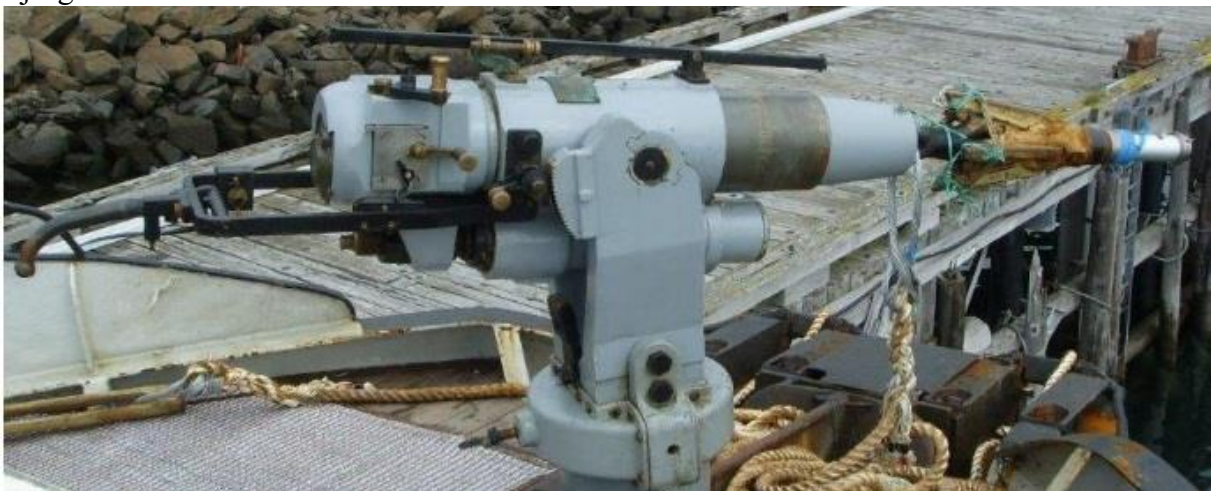
Fig. 3. 90 mm Kongsberg whale cannon with harpoon and modified Hvalgranat-99 ready to fire. Photo: EO Øen Fig. 4.
