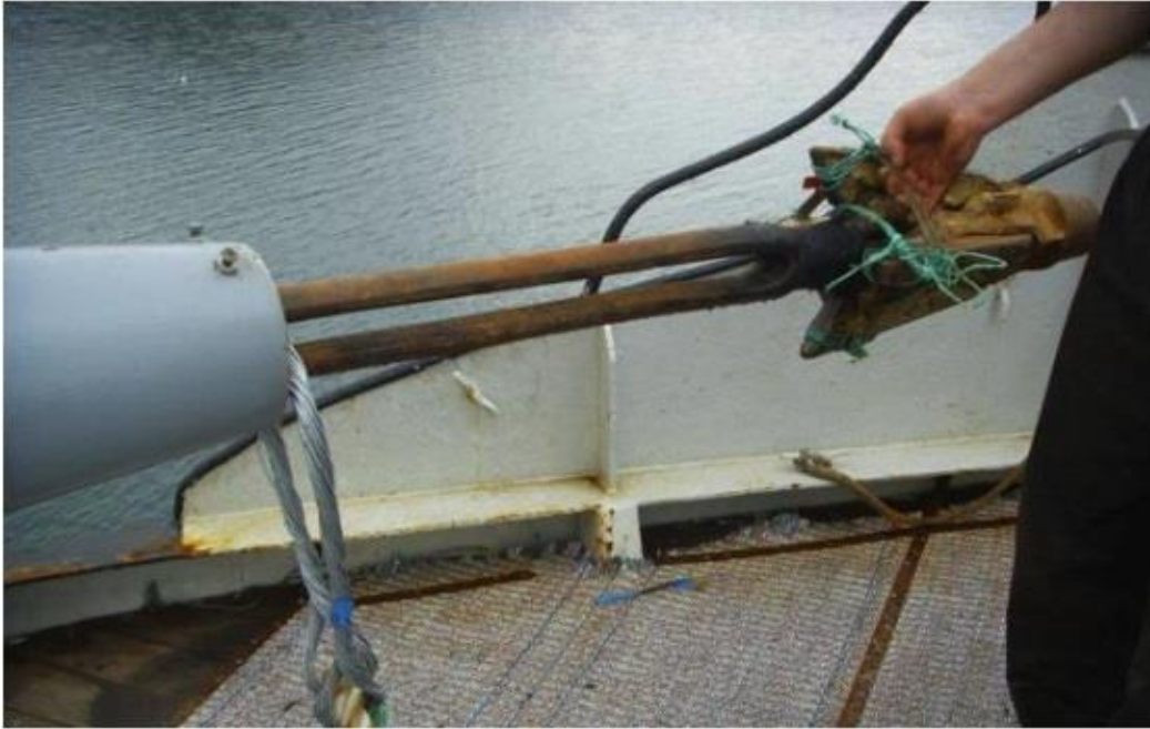
Fig. 17. Harpoon is inserted into the barrel. Photo: K Loftsson
