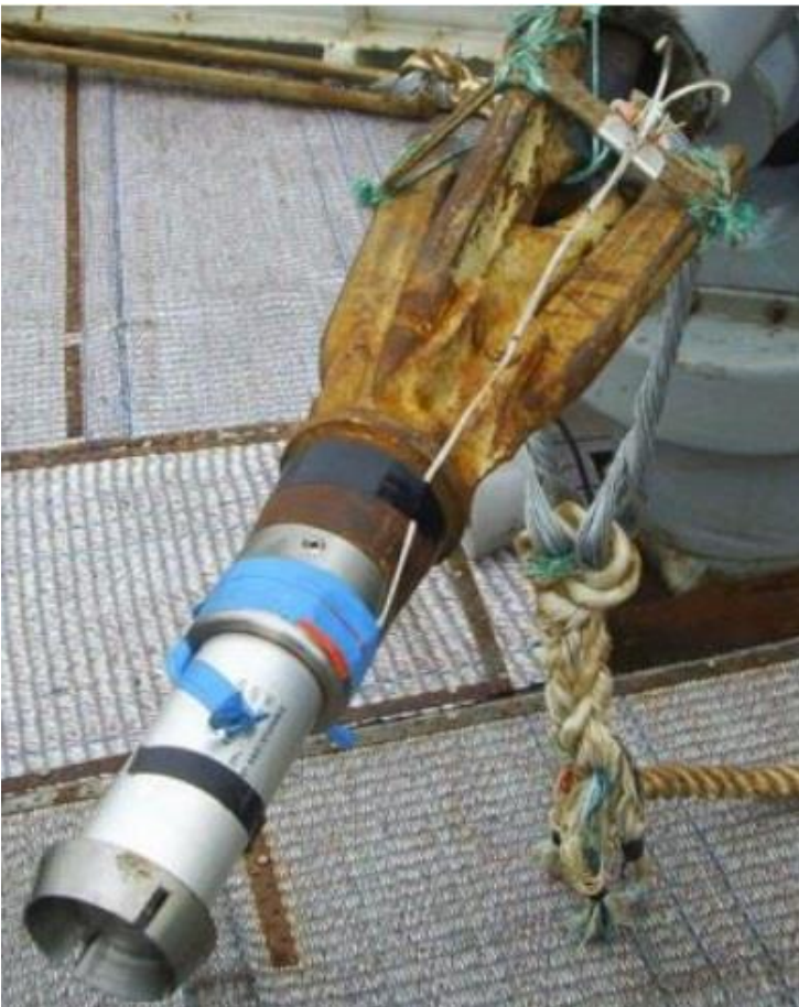
Fig. 18. 90 mm Kongsberg whale cannon with harpoon and modified Hvalgranat-99 for large whales. Trigger hook is attached to the bend sling on the harpoon. Photo: EO Øen
