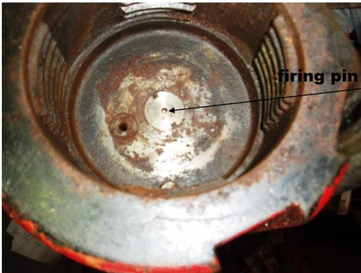
Fig. 5. The buttplate in the breech of the 50 mm Kongsberg whale gun. The firing pin in the rear (secured) position. Photo: EO Øen
