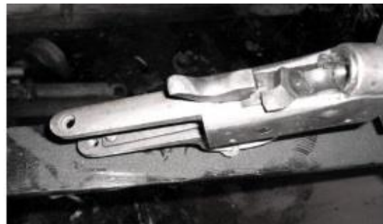
Fig. 23. HHMV ignition mechanism ( blue color) Photo and illustration: EO Øen
