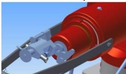
Fig. 23. HHMV ignition mechanism ( blue color) Photo and illustration: EO Øen
