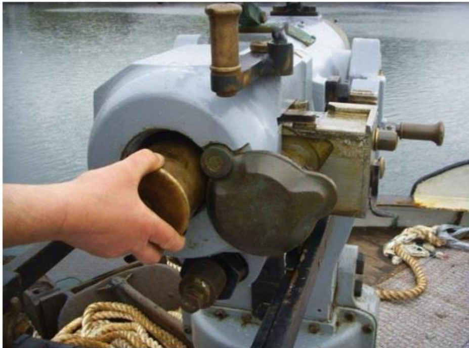
Fig. 12. 90 mm Kongsberg whale cannon with open breech. Photo: EO Øen 3. Check that the shell fits into the chamber (shells expand with use, and must regularly calibrated or replaced) (Fig. 13).
