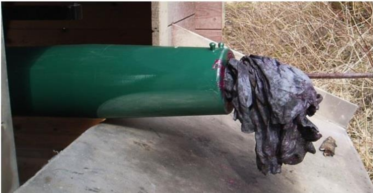
Fig. 19. Cleaning the barrel of a whale cannon. (From firing test). Photo: EO Øen
