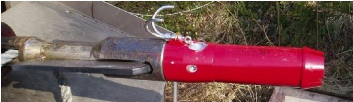
Fig. 27. Whale grenade-99 with trigger hook. (From trial firing of whale shells). Photo: EO Øen
