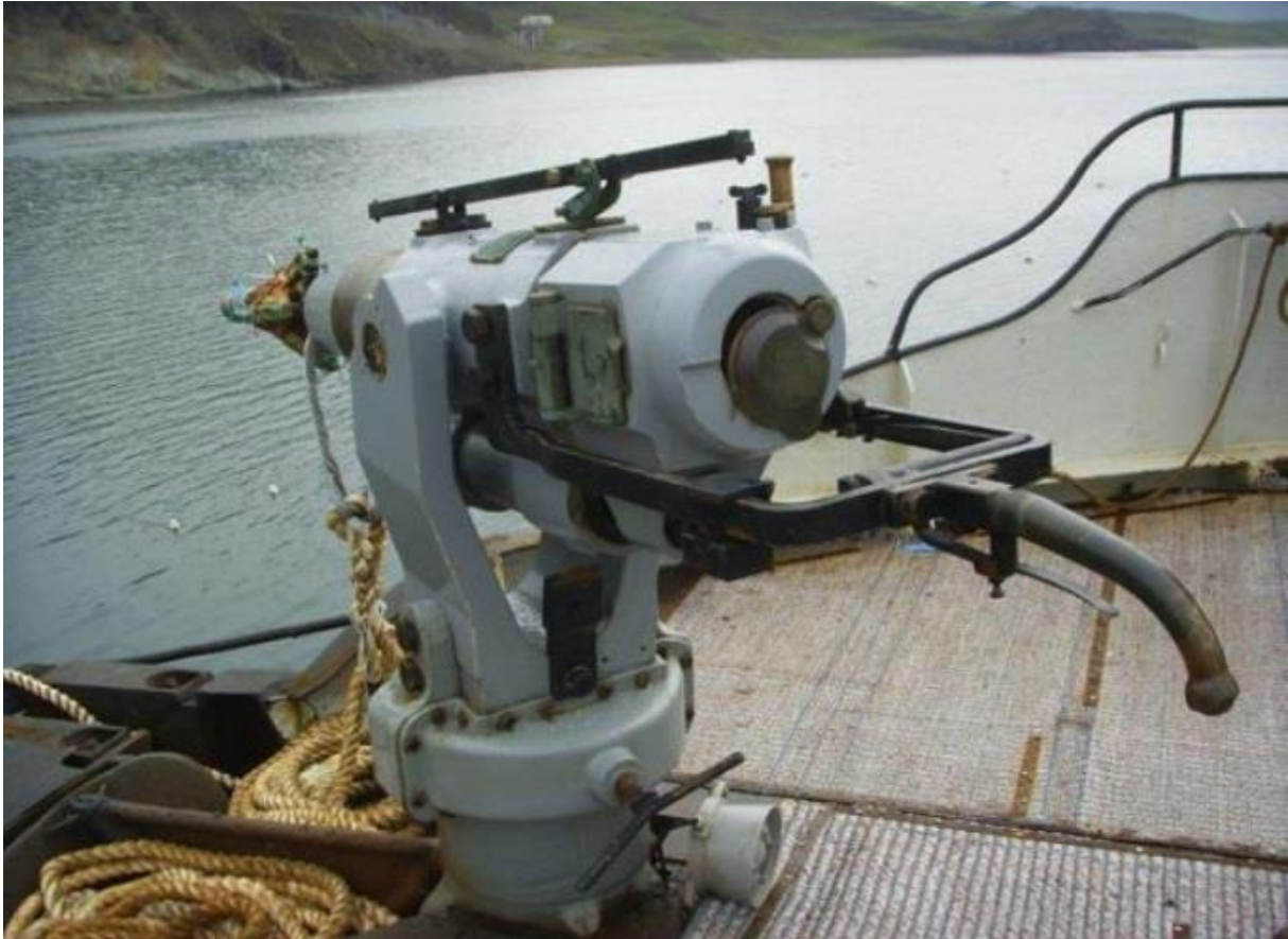
Fig. 11. Fully loaded 90 mm Kongsberg whale cannon. Photo: EO Øen
