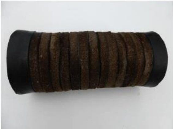
Fig. 14 and 15. Precharging for 90 mm Kongsberg whale cannon. Photo: EO Øen
