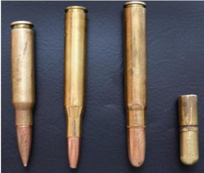
Fig. 38. The figure shows different types of balls. From left: pointed, full-metal cal. 308, lead tip bullet. 30-06, round nose, full mantle cal. 9.3 and round nose, fully sheathed cal. .375. Photo: EO Øen
