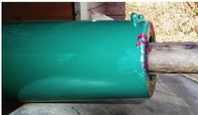
Fig. 22. Powder bag and precharge are pushed in to bottom of the barrel with a charging stick. Photo: EO Øen
