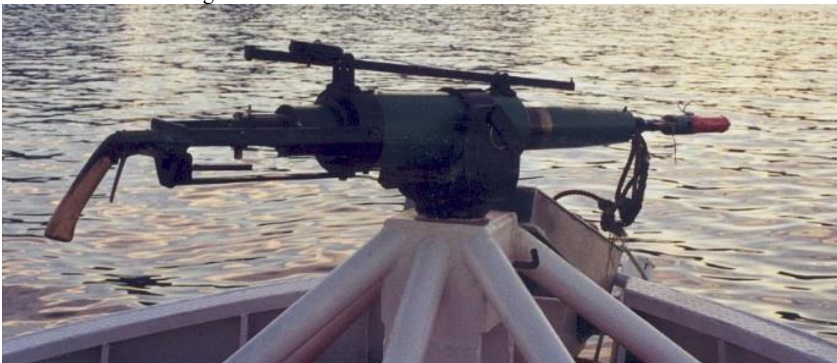
Fig. 3. 90 mm Kongsberg whale cannon with harpoon and modified Hvalgranat-99 ready to fire. Photo: EO Øen Fig. 4.
