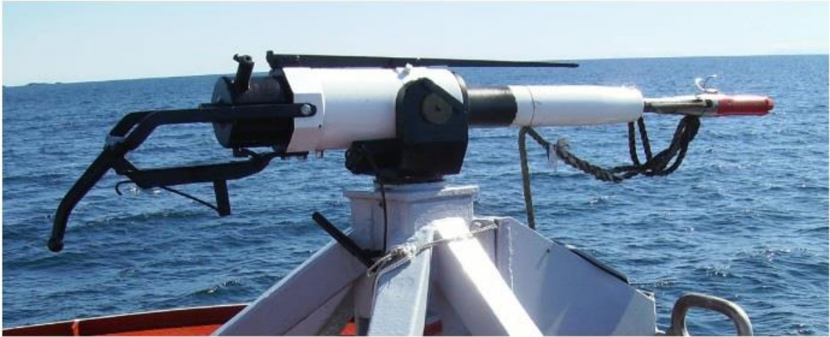
Fig. 2. 50 mm Kongsberg whale cannon with harpoon and Hvalgranat-99 ready to fire. Photo: Björgvin Guðmundsson
