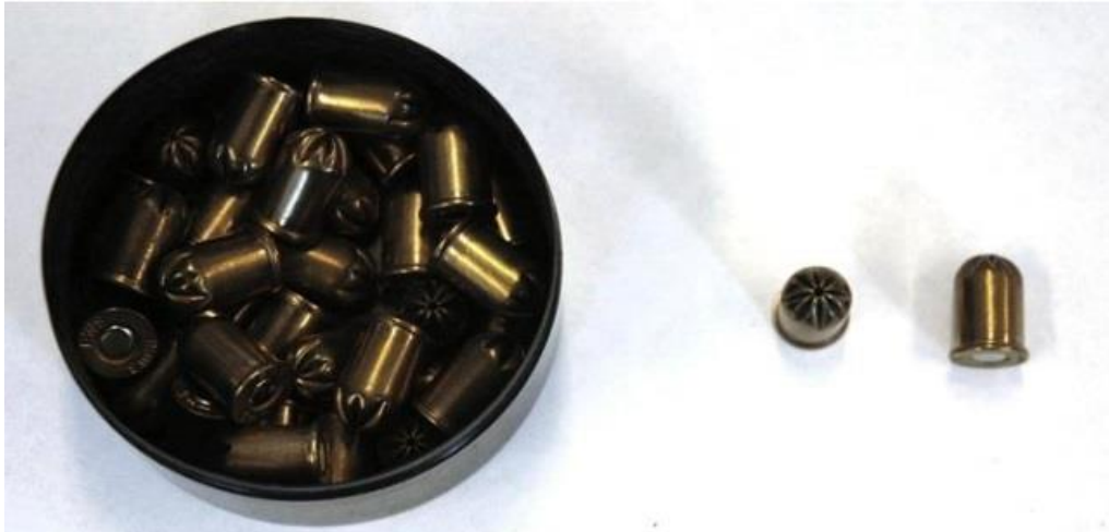
Fig. 8. Example of firing cap/firing cartridge (9 mm) for 50 mm Kongsberg whale cannon shell Photo: Nette Levermann
