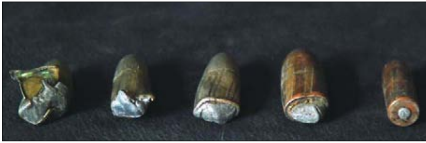
This is what elephant skulls do to bullets (photographed from two angles). Only the .375 on the right penetrated sufficiently.
