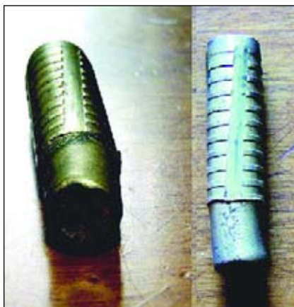
Not all brass monolithics are created equal. These failed on elephant.
