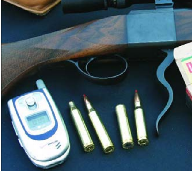
The aftermath of using a cell phone while testing loads – 7mm-08 fired in .25-06 Remington!
