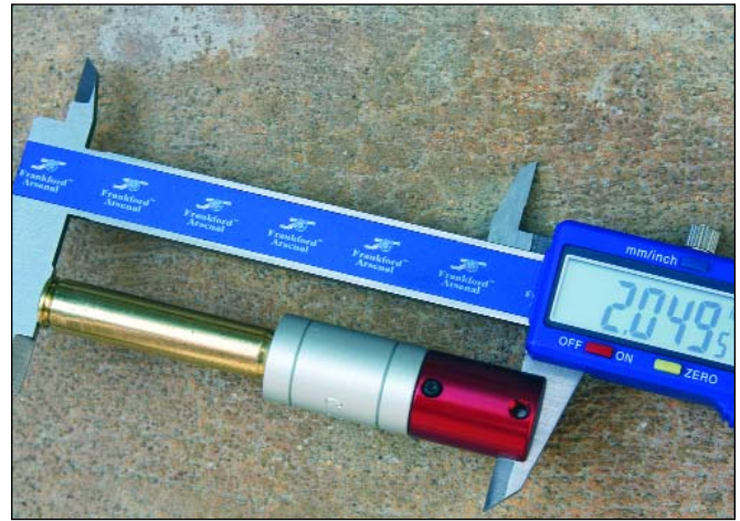
A .25-06 Remington case fired in a Dakota Model 10 after the 7mm-08 had been fired in it indicates no increase in headspacing.
